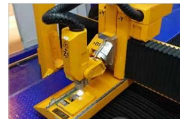
In case MSF Max is equipped with a laser bevel head, the system comes with the ACTG® unit and auto-calibration feature by default. Unlike in other MicroStep machines, the unit is integrated directly into the gantry in a combined calibration station that is ejected during the calibration process. The station contains also a pad for calibration of the capacitive height sensor in the cutting head and a nozzle cleaning system consisting of a camera and a wiping brush.
