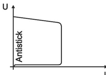
**Anti-stick prevents the electrode from annealing.**
