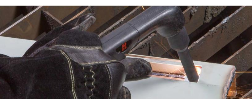
Patented consumables with extra length and a narrower profile for cutting and gouging in hard-to-reach places.
