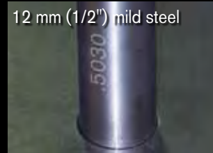
12 mm (1/2") hole with True Hole technology
