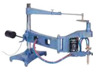
This easy to use machine can reproduce profiles from a reusable steel template. The steel template is traced by a powered magnetic roller with a variable speed SCR control system to provide maximum stability. The template mounting arm is fully adjustable. Templates for internal and external tracing are easily produced by simply incorporating an allowance for the tracing roller diameter and kerf.
