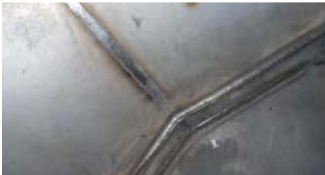
Welding of UNS S32205 in vertical-up and overhead position, using FOXcore 2209-T1.
