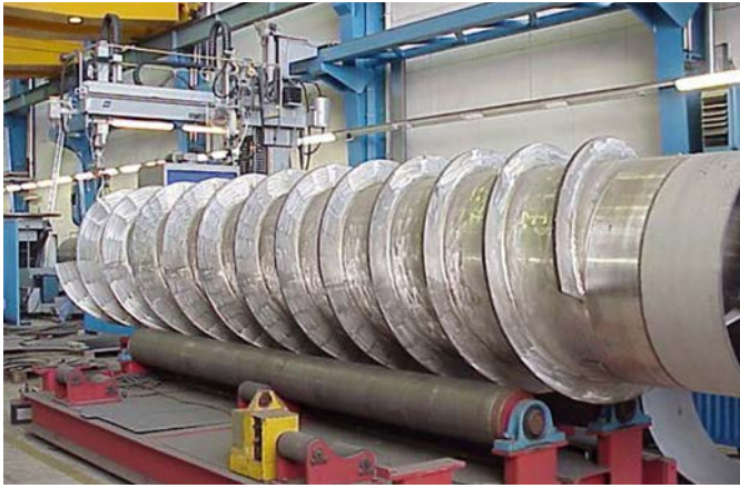
Worm shaft for the pulp and paper industry made of AISI 316Ti and welded with Ø 1.2 mm FOXcore 316L-T0. Courtesy: Andritz AG, Austria.
