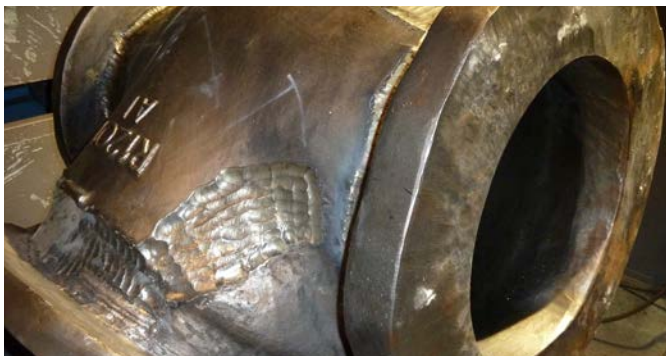
FOXcore 2594-T1 HD used for the repair welding of cast superduplex stainless steel.
