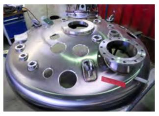
The typical processing time for a complex container bottom machine that allows to process metal sheets as well as dished with many connection parts (as an example see photo above) was about one and a half weeks – today, if required, GEA can
