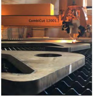
For the jobs at Solintal (e.g. 45° Y-bevels on parts 160 mm thick) oxyfuel was naturally the technology of choice. The movement capabilities of rotator allow to cut a great variety of contour shapes. A high output accuracy is ensured by the possibility of auto-calibration of the oxyfuel rotator – thanks to MicroStep's patented ACTG<sup>®</sup> technology.
