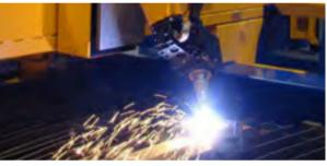
With rotator from MicroStep, V-, Y-, and (under certain conditions) also X- and K-cuts can be produced additionally on already pre-cut parts.
