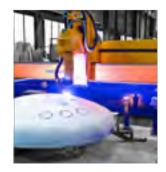
The basic step in production of pressure vessels is precise cutting of tank ends. Automating this process to a high degree while delivering high-precision cutting results without the need of additional surface finishing provides manufacturers with a clear advantage and saves them a lot of valuable time. **P. 20/21**
