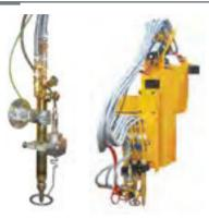
Oxyfuel tool station with manual tilting possibility up to  $\pm 45^{\circ}$ . Fully automatic gas console with preset parameters ensures stable quality of cuts and best efficiency. Multi-tool version enables stripe cutting with stripe width  $\geq$  70 mm.
