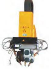
Oxyfuel triple torch with fully automatic gas console enables bevel cutting of V-, plates, pipes, profiles and domes up to 52°. X-, Y- and K-cuts with 3 oxy torches within The innovative ITH torch holder includes bevel range 20° – 50°. Tilting angle and sensors for torch displacement detection, span of torches can be set manually or automatically.
