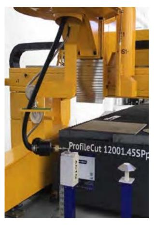
The calibration system ACTG<sup>®</sup> enables durable high-precision results – also with the pantograph. This specialized 3D cutting head with tilting ability of 120° moves around the profile both in the longitudinal and transverse directions.
