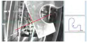
During the scanning process, the real contour of the part is compared with its ideal shape (drawing).
