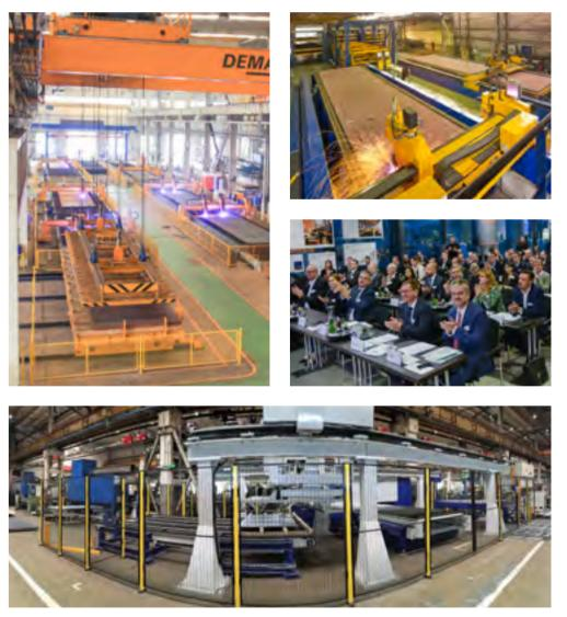
Above right: A production line interconnecting cutting machines with an automatic pallet exchange system and a tower pallet storage for plates allows for 24/7 operation. Above left: CAPP-enabled MicroStep automatic production line uses advanced machine management software MPM to boost production efficiency. In the middle: Representatives of MicroStep at the annual
