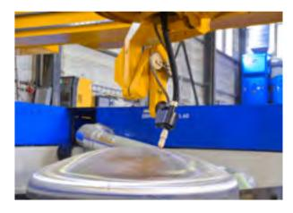
The pantograph plasma rotator with a tilt up to 120° enables weld edge preparation also on the bottom edge of a dome.
