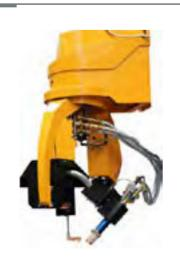
5-axis rotary bevel head with endless rotation enables oxyfuel bevel cutting of plates, pipes and profiles up to 65°. The innovative ITH torch holder includes sensors for torch displacement detection, IHS and auto-calibration.
