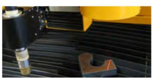
ABP scanner determining the exact position of a part placed on a random spot on the cutting table.
