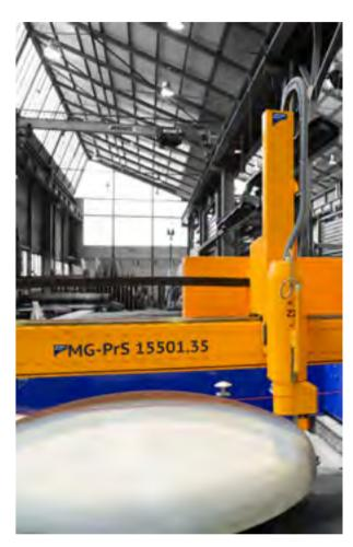
Maximum precision in dome cutting is made possible by MicroStep's mScan technology. In the process, a laser scanner integrated into the portal determines the 3D surface geometry of the workpiece in advance.
