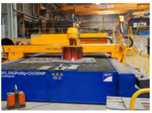
MicroStep delivered the complete cutting solution: with a 12 x 3 m large cutting area for plates up to 150 mm thick and a zone for cutting pipes with a robot situated along the outer side of the machine guides, the machine is capable of processing tubes up to  $\emptyset$  2000 mm and wall thickness 80 mm.
