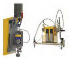
Waterjet tool station for cutting of all types of materials. Multi-tool version can carry up to 4 water jets on a single Z lifter.
