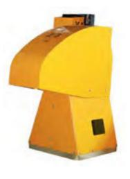
Laser scanner dedicated for scanning of both the contour and position of a straight pre-cut part in ABP feature – additional cutting of bevels for weld edge preparation. ABP technology is available for plasma, laser, oxyfuel and waterjet cutting technologies.
