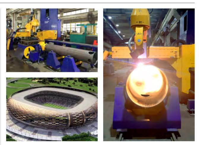
**Top left + right:** Gree's combined pipe & dome cutting machine PipeCut allows to cut pipes up to  $\emptyset$  610 mm and a length of 12 m as well as domes up to  $\emptyset$  1,200 mm. **Bottom left:** Gree Electric Appliances Inc. was chosen to participate on prestigious projects such as the National Stadium (Soccer City) in South Africa's Johannesburg.
