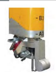
5-axis rotary bevel head for waterjet enables bevel cutting of all types of materials up to 45°. Adaptive taper compensation (ABC) and periodic height sensing (PHS) are included by default.
