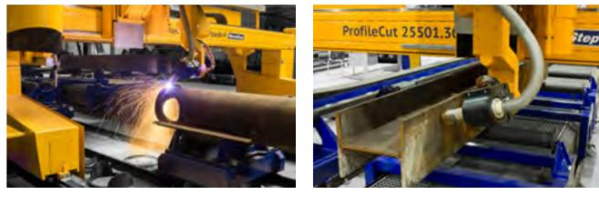
MicroStep has developed a variety of solutions for high-precision 3D processing of tubes, profiles and beams – including fully automated material handling.
