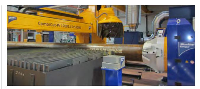
ables bevel cutting up to 50° on both plates and pipes. "We used to buy pipes from a supplier. The problem was that it was very inflexible – deliveries took too long," says Pierre Ruble.
