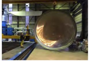
When designing the plasma cutting machine, the focus was on the precise and flexible processing of domes. A special dome cutting table supports domes from 500 mm up to 5,500 mm in diameter.
