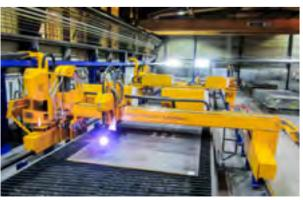
The combined plasma and oxyfuel cutting solution at MAP Prinzing Brennschneidtechnik GmbH enables bevel cutting with plasma, 2D oxyfuel cutting, drilling, tapping and marking on two gantries. At the request of the company, a tool magazine for 16 tools was added.
