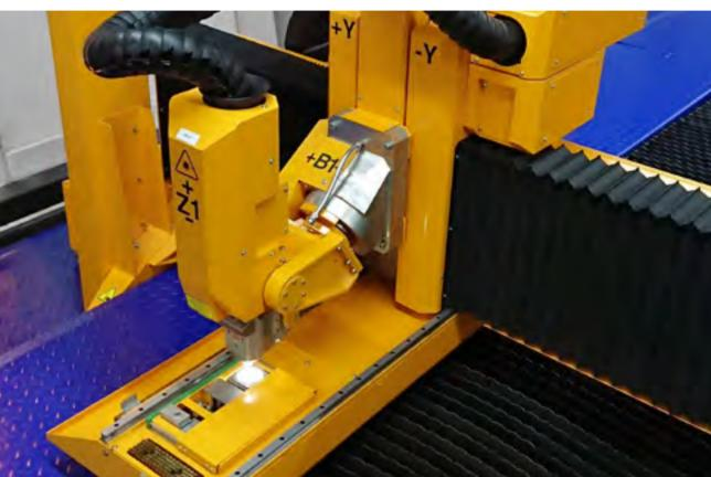
**Above:** Chantiers de l'Atlantique opted to invest into a large-scale fiber laser cutter MSF Max. It is a 50 m long machine with two 21,000 x 3,500 mm cutting zones.
