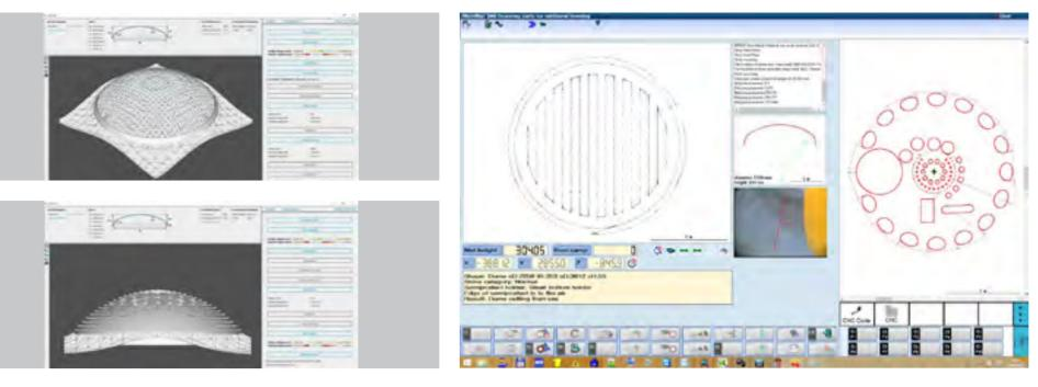
Thanks to the mScan technology, the 3D scan of a dome enables to determine production-related deviations from the ideal contour that then could be compensated for accordingly during cutting.
