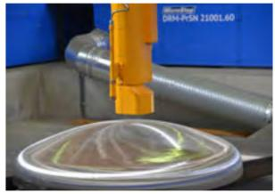
The laser scanner can reach the entire dome surface. The measured data are compared with the ideal dimensions on which the cutting plan is based and deviations are automatically compensated for during the cutting process.
