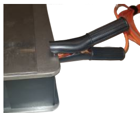
Figure 48: Workpiece clamp connected to electrically conductive welding table
