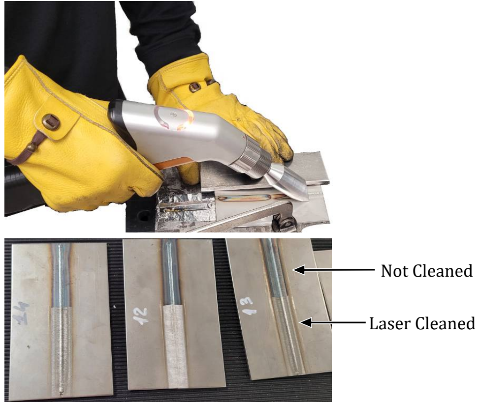
Figure 49: LightWELD Operator Performing Laser Cleaning
