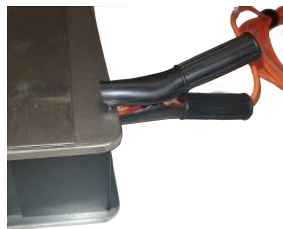
Figure 46: Workpiece clamp connected to electrically conductive welding table
