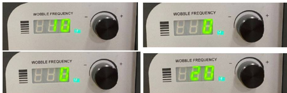
Figure 32: IP Address shown at first power up after AC line cord is plugged into an outlet
