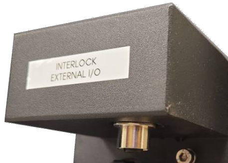
Figure 24: 12-pin M12 Female Interlock External I/O Connector, A Orientation
