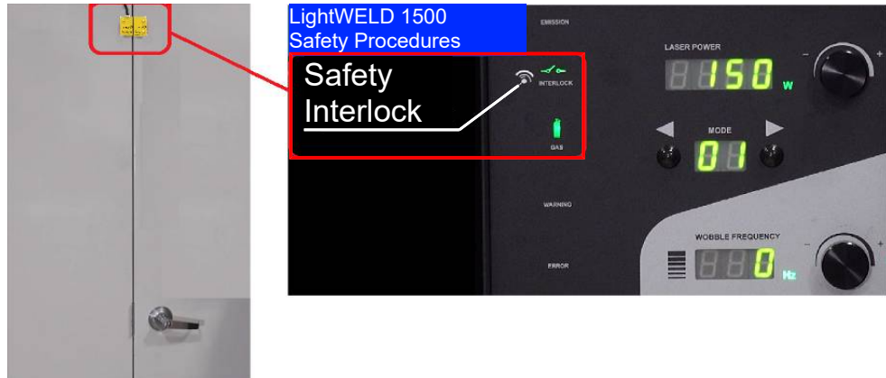
Figure 31: Door Interlock Closed - Safety Interlock is Satisfied
