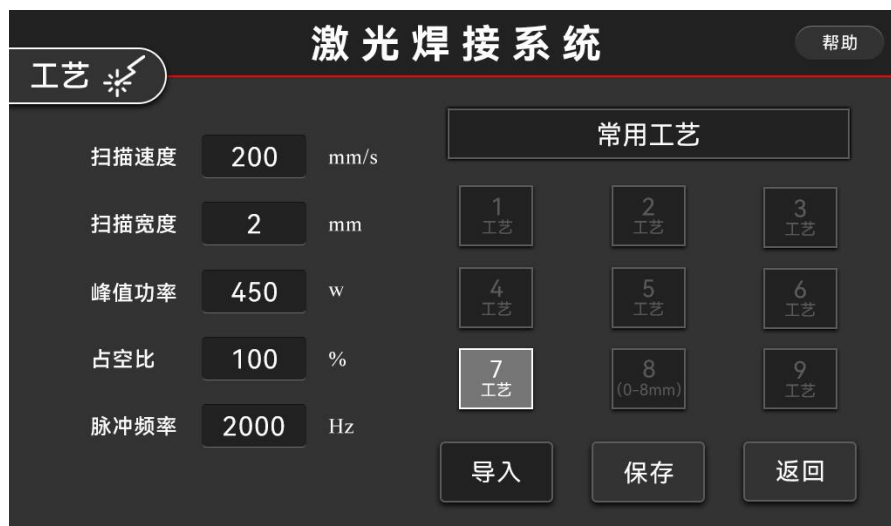
Figure 3-2 Process interface on the control panel
