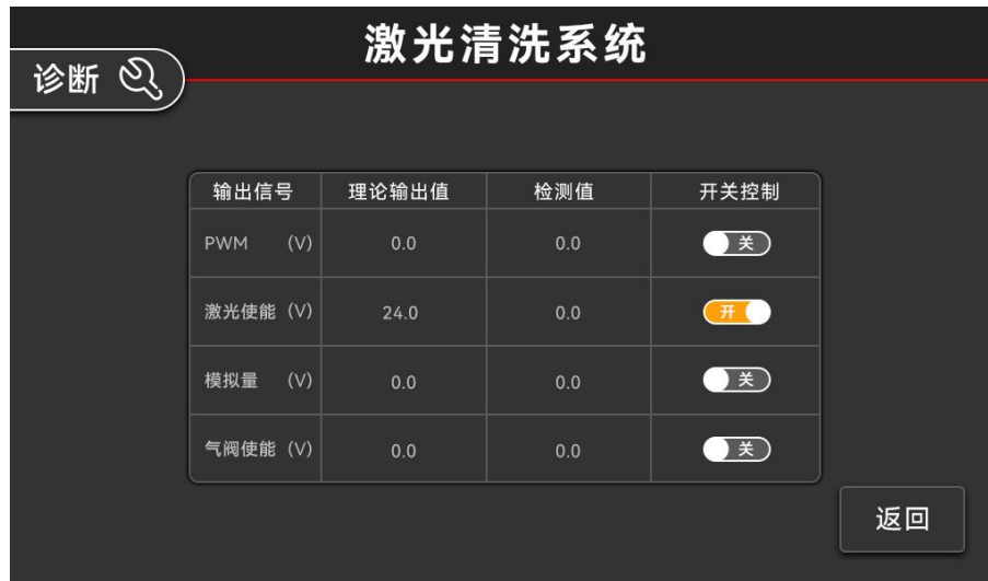
Figure 3-24 The diagnosis interface of laser cleaning system
