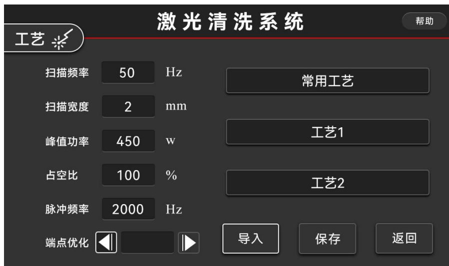
Figure 3-19 The process interface of professional cleaning system
