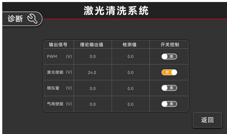
Figure 3-14 The diagnosis interface of laser cleaning system
